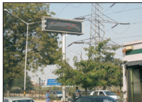
Fig. 6: VMS at Madanpur Khadar Junction
